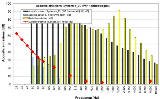
Acoustic emissions of supply duct of the unit Systemair Genius [dB]
