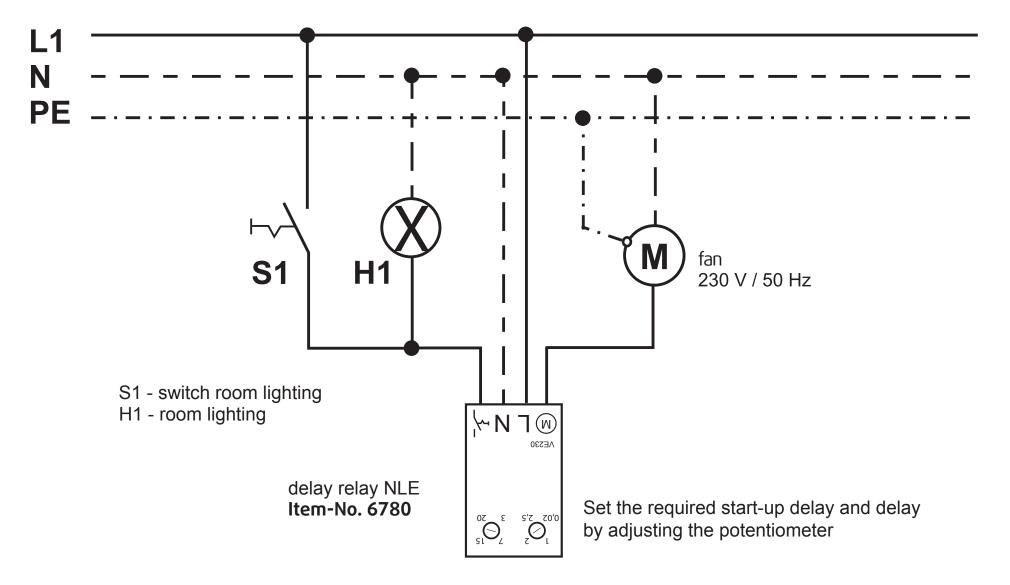
The electrical connection must be performed by a specialist according to VDE 0100. During intallation and assembly work an all-pole disconnection must be made from the mains with a minimum 3 mm contact opening width.
