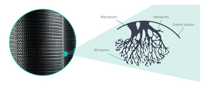
To prevent grease and other solid particles from blocking pores on the surface of the activated carbon filters and to increase the lifetime of the system, the activated carbon filters should always be placed after fine filtration (electrostatic precipitator, bag and/or HEPA filter) grades. Otherwise, the activated carbon filter may lose its odour-removing capabilities in a shorter period of time.
