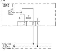
Max. Schaltstrom / max. switch. current Klemmen / terminal 5-2: 3(1)A 250V AC Klemmen / terminal 5-1: 10(3)A 250V AC
