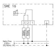
Max. Schaltstrom / max. switch. current SGTS02K0 Klemmen / terminal 1-3: 16(4)A 250V AC, 10(4)A 400V
