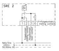
Max. Schaltstrom / max. switch. current 10(3)A
