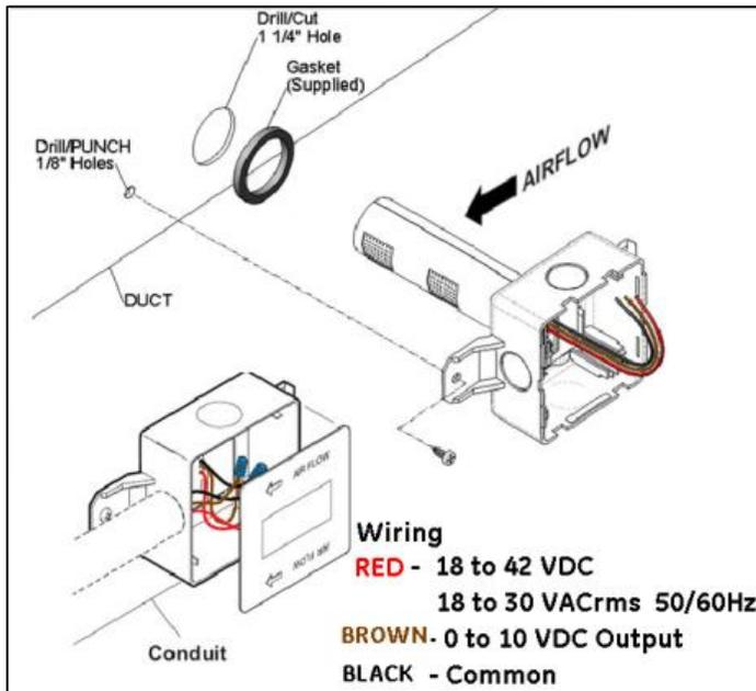
Figure 1: Systemair-1 CO<sub>2</sub> duct sensor Installation
