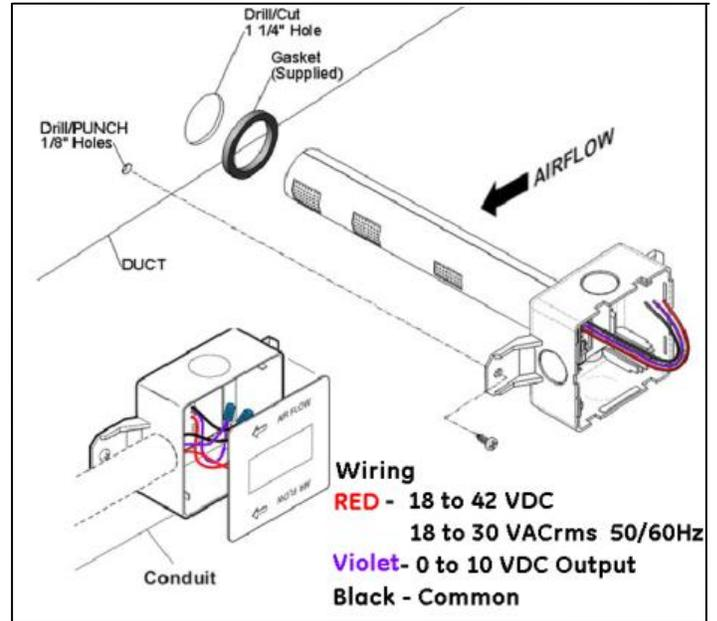
Figure 2: Systemair-2 CO<sub>2</sub> duct sensor Installation
