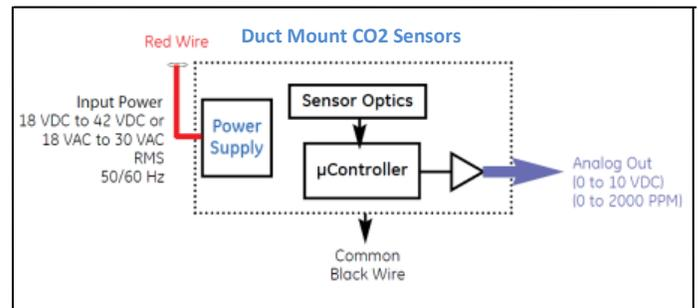
Figure 3: Wiring
