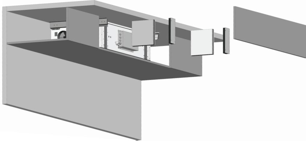
**Utrustning utdragen, inspekionslucka öppen | Pulled out unit, inspection door open**
