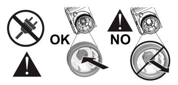
Figure 5: Spindle retracted
