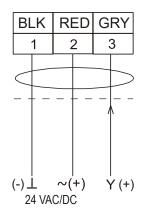
Figure 11: 24 VAC/VDC Proportional Model
