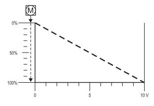
Figure 15: The dip switch 4 OFF (Direct Acting – DA) When the signal increases the actuator stem extends.
