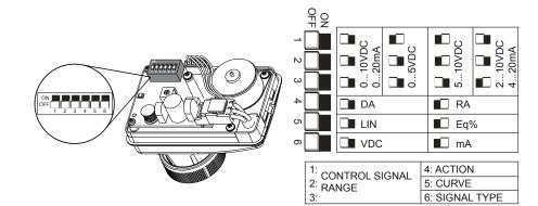
Figure 13: VA-7482 dip switches
