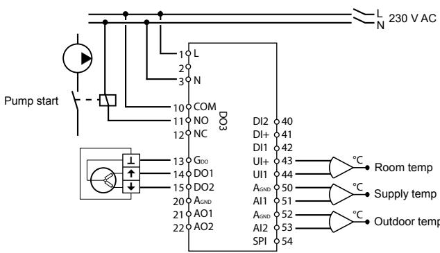
Figure 3. Wiring example: OP10-230 with 3-position actuator and room temperature sensor (can also be used without a room temperature sensor).
