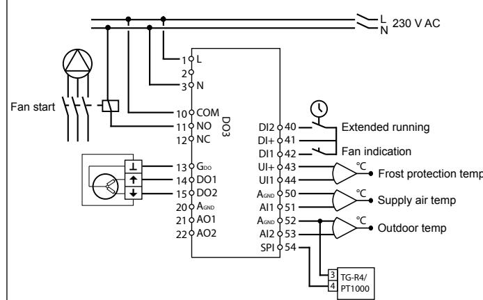
The digital outputs are 24 V AC, G<sub>0</sub> is common and DO is connected to G<sub>0</sub>. For OP10, DO1 and DO2, the outputs can handle 12 VA. For OP10-230, DO1 and DO2, the outputs can handle 3.8 VA when using the internal transformer.
