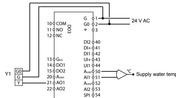
Figure 4. Wiring example: OP10 with 0...10 V actuator
