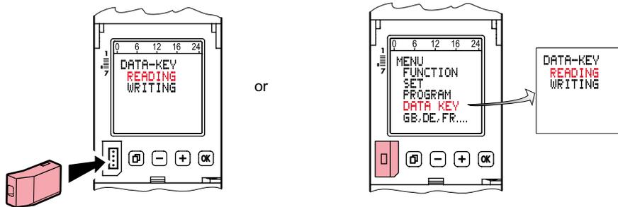
Load the programs from the data key to the time switch (READ KEY)
