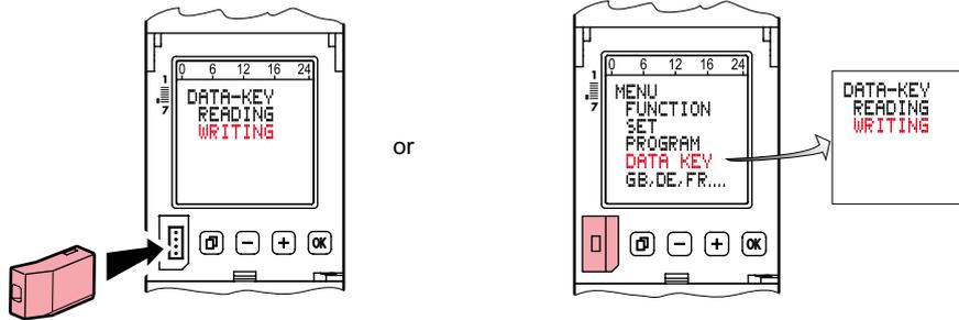
Load the programs of the time switch on to a data key (WRITE KEY)
