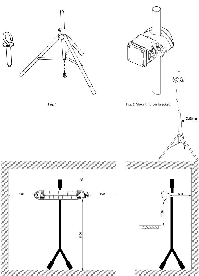
Fig. 3 Minimum mounting distance
