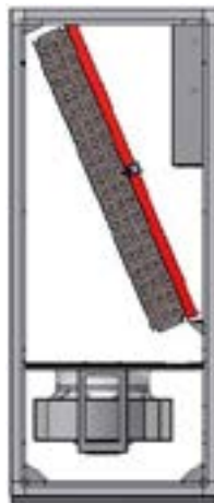
Position P unit air filters with air supply facing downwards
