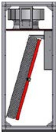
Position P unit air filters with air supply facing upwards
