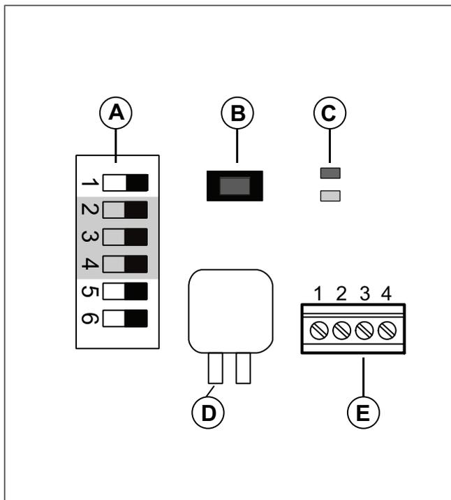
Figure show dip-switches to the left, position OFF.
