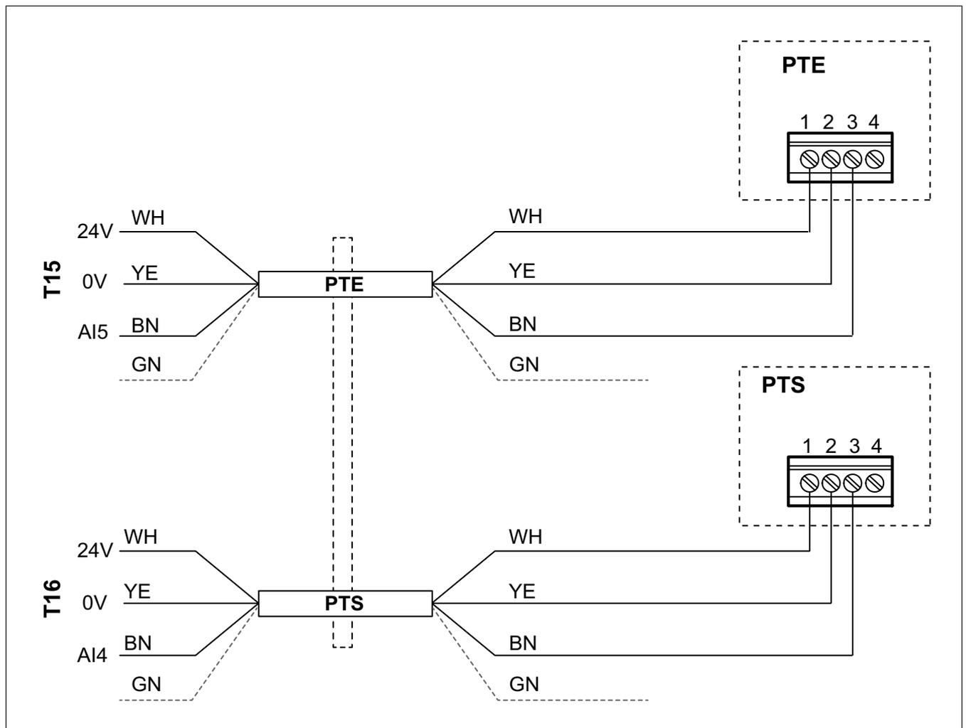
Green cable should not be used. Isolate to avoid short circuit.
