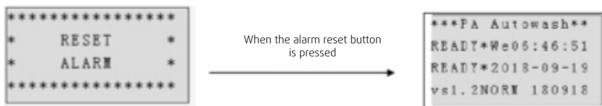
Figure 29: The alarm reset procedure and the text displayed on the PLC screen
