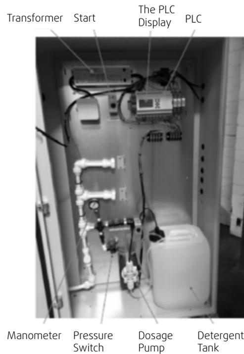
Figure 24: Internal setup of the Autowash system
