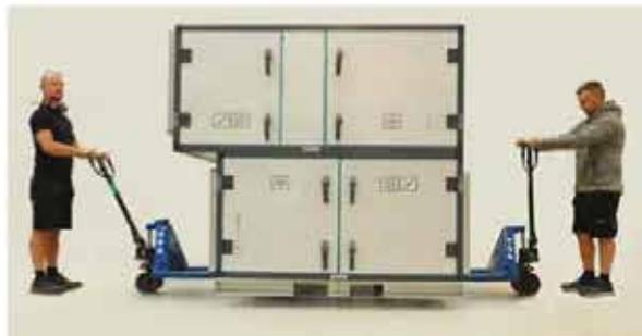
Figure 7. Lifting with Pallet Truck
