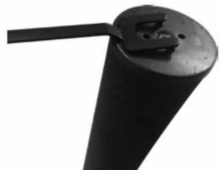
Figure 20: Mounting apparatus for the active carbon filter
