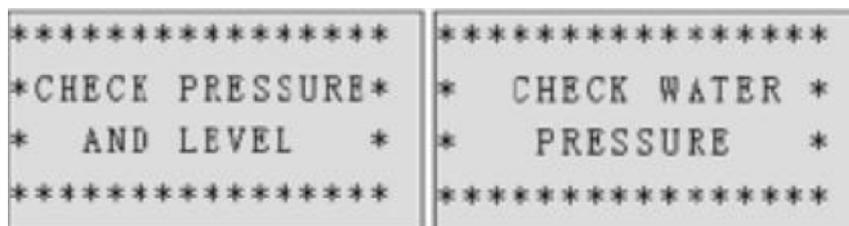
Figure 28: Reading the reason for the blue alarm light being on from the PLC screen
