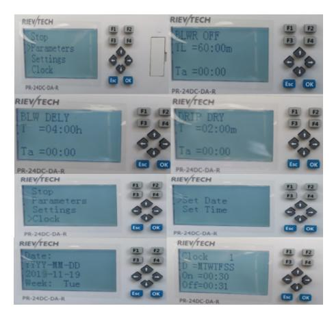
Figure 32: Reprogramming the washing period over PLC
