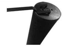
Figure 20: Mounting apparatus for the active carbon filter
