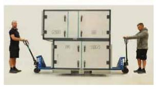
Figure 7. Lifting with Pallet Truck
