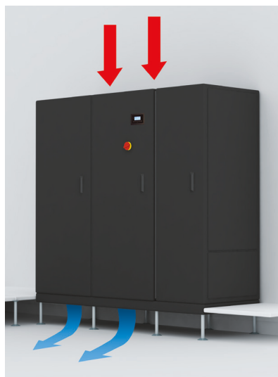
Standard version with top air intake and downflow air supply, with stand for raised floors.
