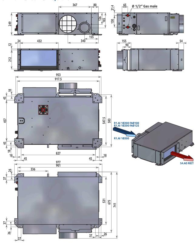
CONFIGURATION R2.AI 1Ø200/S4.AO RECT OR R2.AI 1Ø200 FAØ100/S4.AO RECT OR R2.AI 1Ø200 FAØ125/S4.AO RECT
