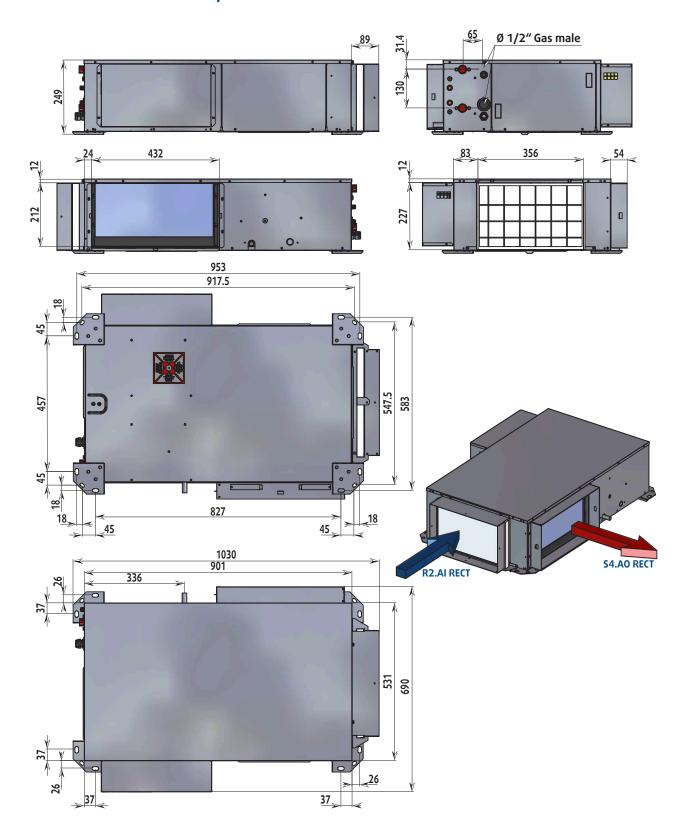
CONFIGURATION R1.AI 1Ø200/S4.AO RECT OR R1.AI 1Ø200 FAØ100/S4.AO RECT OR R1.AI 1Ø200 FAØ125/S4.AO RECT
