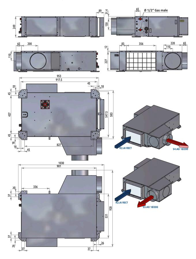
CONFIGURATION R1.AI 1Ø200/S4.AO 1Ø200 OR R1.AI 1Ø200 FAØ100/S4.AO 1Ø200 OR R1.AI 1Ø200 FAØ125/S4.AO 1Ø200 OR R1.AI 1Ø200/S3.AO 1Ø200 OR R1.AI 1Ø200 FAØ100/S3.AO 1Ø200 OR R1.AI 1Ø200 FAØ125/S3.AO 1Ø200
