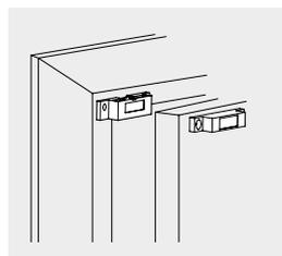
MDC, magnetic door contact with time relay
