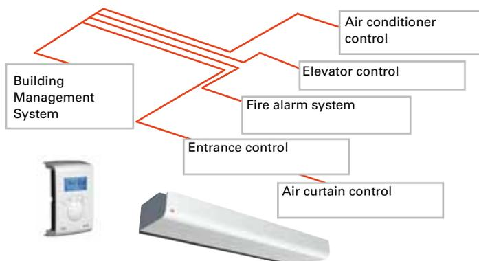
Integration of Frico air curtains in an overall control system (BMS)
