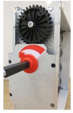
The damper blades are fitted with synthetic bearings requiring no lubrication. Air-tightness of the damper, when the damper motor is in the closed position, must be visually checked once a year. The damper motor is to be adjusted if the damper does not close tightly.
