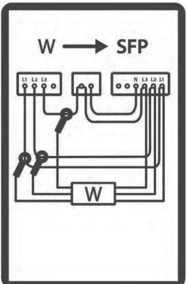
With removed cover called service door in the inspection door there is free access to place ampere measuring clamps around the cables and free access to terminals to measure volt.
