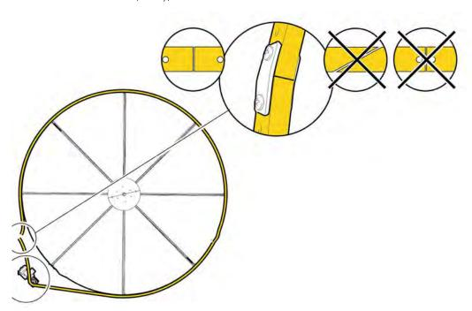
Check the drive belt annually. Replace if necessary. Reuse both brackets. If new screws are needed do not hesitate to make the screws even with the surface of the inner bracket.
