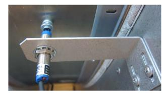
Check the illustrated screw on the rotor for activation of signal from the sensor.
