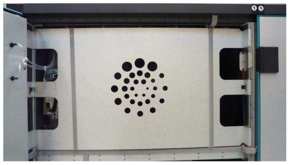
Use an Allen key - size 6 or size 8 - for refitting the safety guard from Systemair. Replace the vibration damping rubber list if it is damaged.
