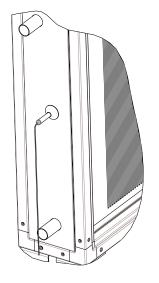
Coil seen from above. The sensor measures the water temperature of the water inside one of the small pipes for return water in the coil. The sensor reduces the area in this pipe and hereby also the flow of warm water in this pipe. The temperature in this pipe is reduced more than the temperature in all other pipes by the airflow through the battery. Because the lowest temperature in the battery probably is measured here, this system creates early and safe warning of frost.
