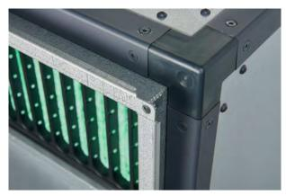
Use 8 mm bolt with nut in each corner and a sufficient number of screw clamps with a distance between screw clamps that not exceeds 300 mm to hold the duct, damper, coil or attenuator tight together
