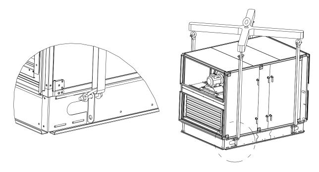
Lifting beam and straps are not included in the delivery.
