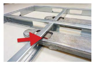
The forks of the manual hydraulic hand truck must be longer than the width or length of the section/unit to achieve safe transport of the section/unit.
