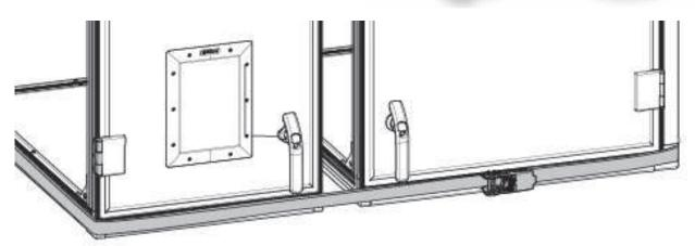
Note! Place the strap on the bottom profiles of the unit to avoid any load and stress on the vertical profiles when sections are pulled together along the base frame or on the floor. The sections must be pulled fully and tight together with the strap placed on the bottom profiles.
