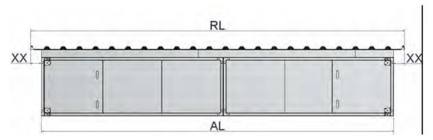
In the table below you will find 40 different lengths of roofs (always changing with the 205 mm) and the lengths of units that are ideal for each of the 40 alternative roof lengths.
