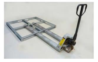
Do not activate the wheels of manual hydraulic hand truck on the horizontal profile of a middle profile. Activation of the wheels on the horizontal profile might bend the profile.
