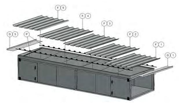
Squeeze sealant in sufficient quantity between the underside of the rails A1, B2, C3, D4, E5 and the horizontal top side of the unit before the rails are mounted. This means that the rails are standing on sealant to achieve the tightest
