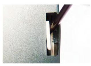
5 Grip the battery firmly with your fingers and lift it upwards until it rises from its holder. Press the new battery firmly down into place. Note that to preserve correct polarity; the battery can only be inserted the "right way round".
