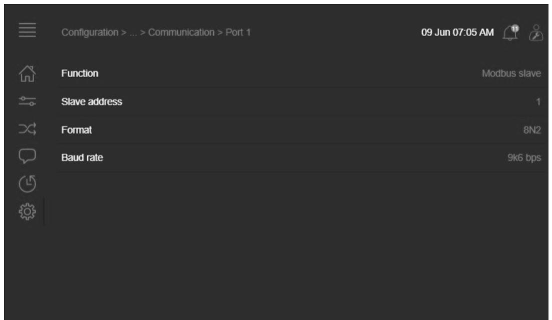
The communication parameters for the Modbus line is the most important thing to configure first. These parameters must be identical in both the master unit and slave units, since they define the structure of messages and the transmission speed.
