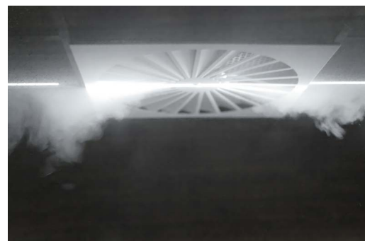
Fig. 2: Cold air supply (< 18°C)
