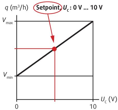
$$U_c = \frac{q - V_{\min}}{V_{\max} - V_{\min}} \cdot 10$$
