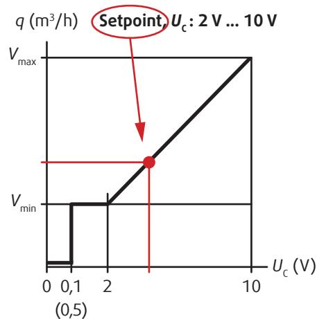
$$U_c = 2 + \frac{q - V_{\min}}{V_{\max} - V_{\min}} \cdot 8$$
