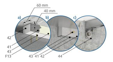
**F1** Screw ≥ 5,5 DIN7981 or suitable wall plug and screw size 6.
