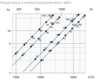
Pressure drop & A-weighted sound power level in dB(A)
