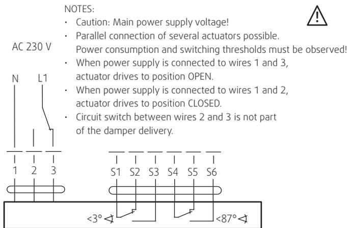
Fig. 3: Connection of the actuator BELIMO BLE 230
