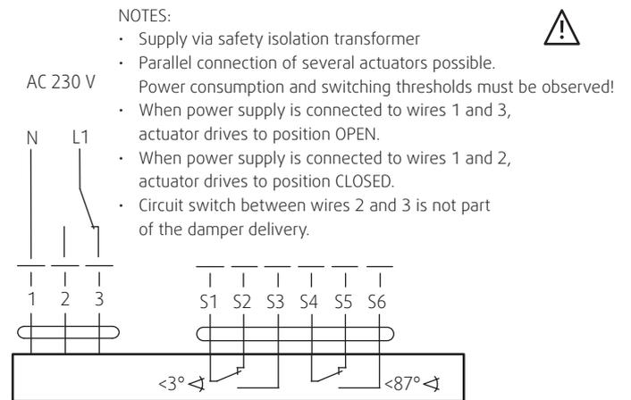
Fig. 4: Connection of the actuator BELIMO BE 230-12
