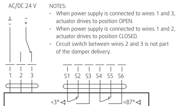
Fig. 6: Connection of the actuator BELIMO BE 24-12-ST
