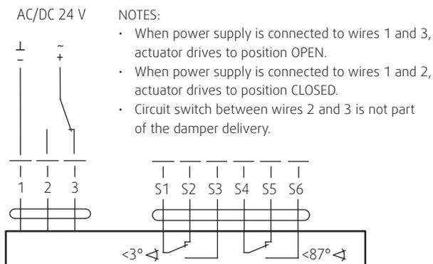
Fig. 5: Connection of the actuator BELIMO BLE 24
