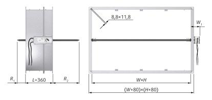
Fig. 10: Dimensions of the rectangular smoke damper with W > 1200 mm up to  $1500 \times 800$  mm NOTE: These smoke dampers have flanges width 40 mm.
