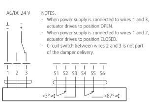
Fig. 5: Connection of the actuator BELIMO BLE 24
