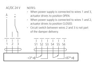
Fig. 6: Connection of the actuator BELIMO BE 24-12-ST
