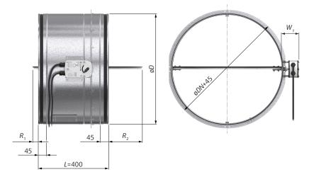
Fig. 8: Dimensions of the round smoke damper
