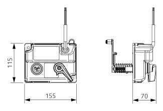
Fig. 4: Dimensions of the manually operated activation mechanism
