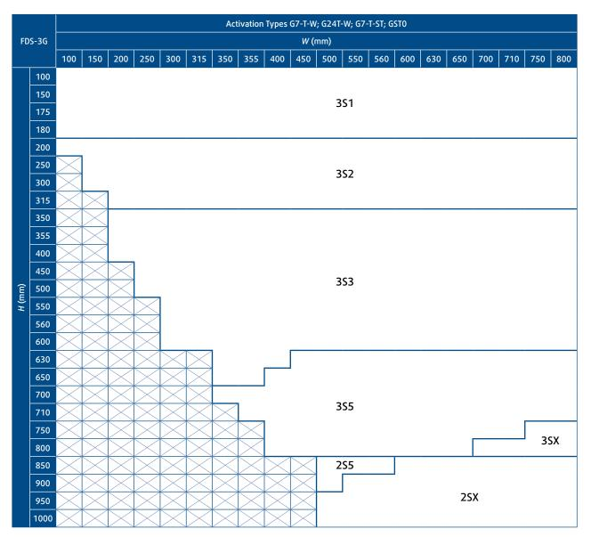
Tab. 7: (part 2/2) Compatibility code for the FDS-3G rectangular fire damper with Gruner actuator operated activation mechanisms plus preparation for communication unit or plus the communication unit itself
