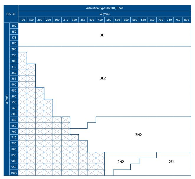
Tab. 4: (part 2/2) Compatibility code for the FDS-3G rectangular fire damper with Belimo actuator operated activation mechanisms
