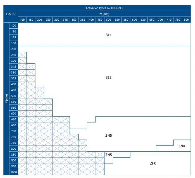
Tab. 6: (part 2/2) Compatibility code for the FDS-3G rectangular fire damper with Gruner actuator operated activation mechanisms
