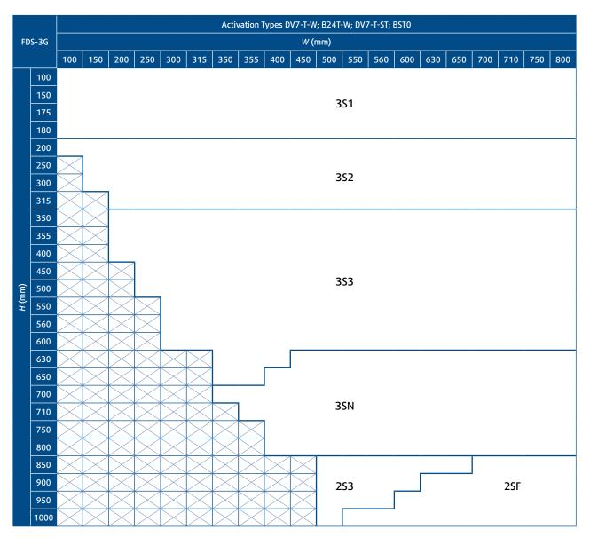
Tab. 5: (part 2/2) Compatibility code for the FDS-3G rectangular fire damper with Belimo actuator operated activation mechanisms plus preparation for communication unit or plus the communication unit itself
