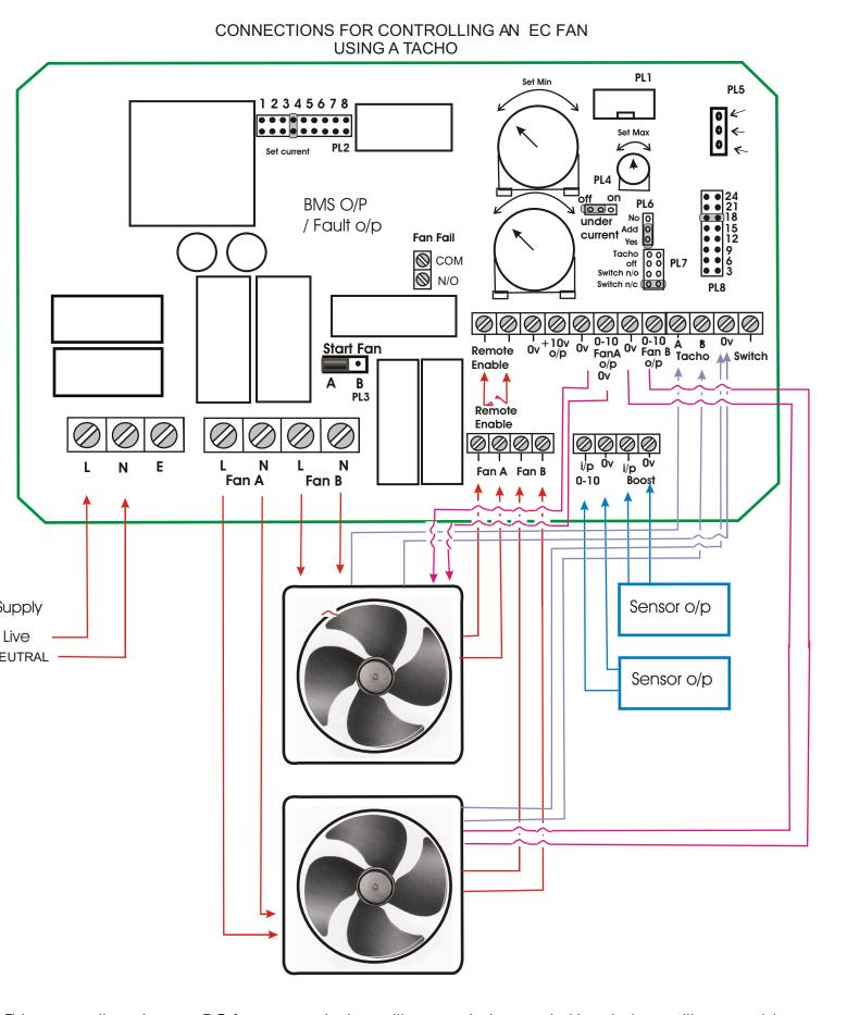
This connection shows a DC fan connected up with a zero to ten control input along with an enable .
