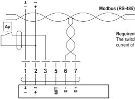
Requirements for switching contact: The switching contact must be able to accurately switch a current of 16 mA at 24 V.
