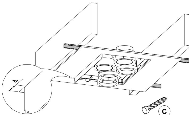
Screw anti-vibration brackets with a ceiling mounting kit to the main ceiling. Use included screws (C).
