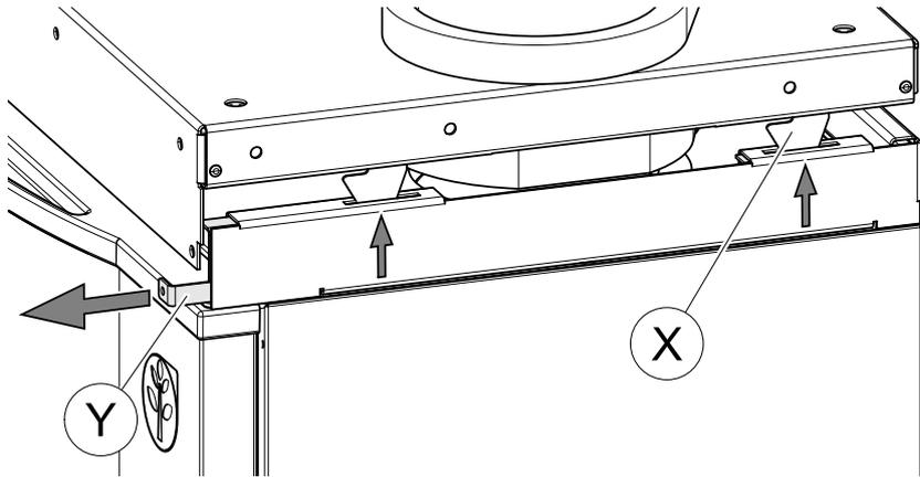
Lock hooks (X) should go through brackets. Pull out the lock mechanism (Y) if needed.
