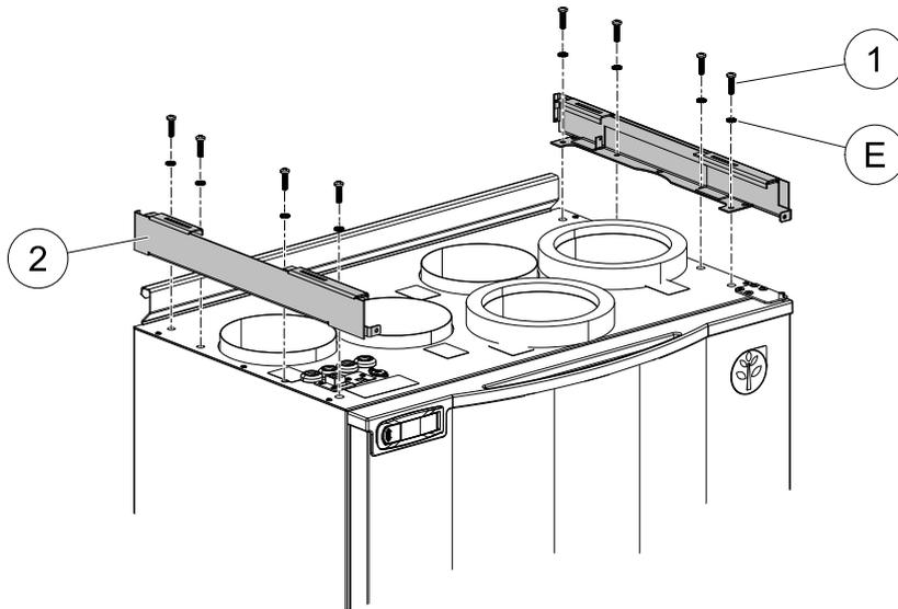
Loosen 8 M5 screws (1) on both sides of the unit. Attach side brackets (2) that came with ceiling mounting kit and secure them with the same screws (1) and included washers (E).
