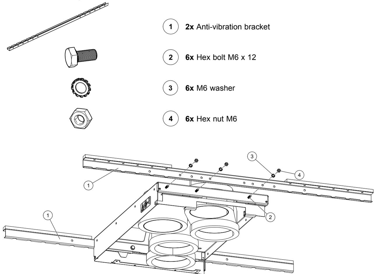
Anti-vibration brackets (1) should be screwed to the ceiling mounting kit from both sides with added hex bolts (2) and tightened with washers (3) and hex nuts (4).
